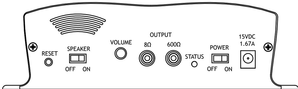
RESET - The RESET button clears audio stored on memory when held during power up. Note: Audio is automatically erased when changing CD media.
